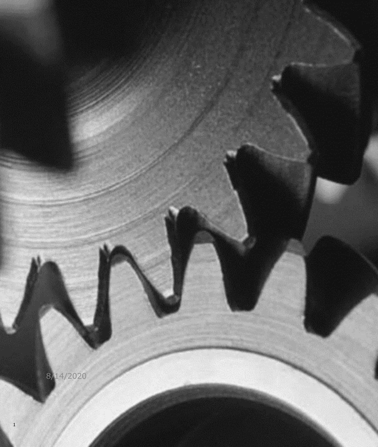
A close-up, black and white photograph of a large industrial gear. The gear has several teeth, and a prominent crack is visible on the surface of one of the teeth, extending from the tip towards the base. The lighting creates strong shadows and highlights, emphasizing the texture and the damage.
